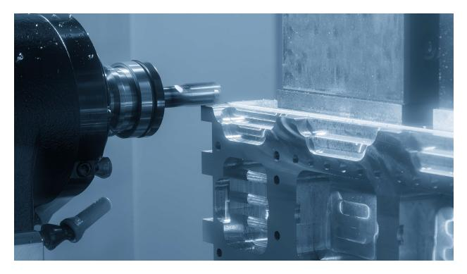
Most customers don't care how their parts are machined as long as they are done economically, correctly, and on-time. But more sophisticated buyers do care because they understand the inherent differences between vertical versus horizontal milling. And they know that no one size fits all, meaning that the characteristics of a specific part will largely determine the optimal type of CNC machine for the job at hand.
