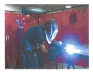
Also referred to as Gas Metal Arc Welding (GMAW), MIG -- an abbreviation for Metal Inert Gas -- is a semi-automatic welding process that feeds a consumable, which is the wire, onto the workpiece. TIG, which stands for Tungsten Inert Gas, and can sometimes be called Gas Tungsten Arc Welding (GTAW), is a manual welding process that uses a non-consumable tungsten electrode to produce the weld.
