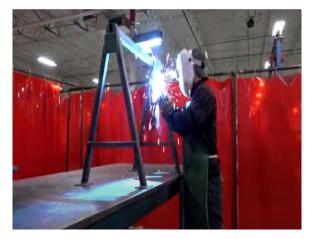
be artistic. With TIG, welders have full control over the amount of heat and the penetration level of the bead. They can also start and stop in any position and don't have to worry about impurities.
