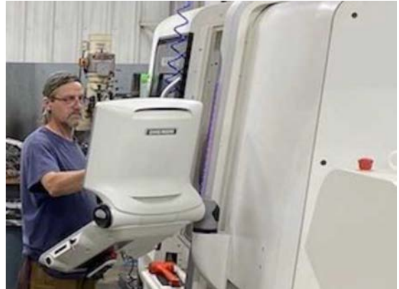
Figure 2: DMG Mori multitasking mill/turn machine at Advanced Machining.
