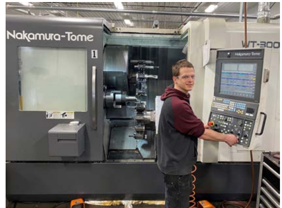
Figure 1: Nakamura-Tome multitasking mill/turn machine at Douglas Machining.
