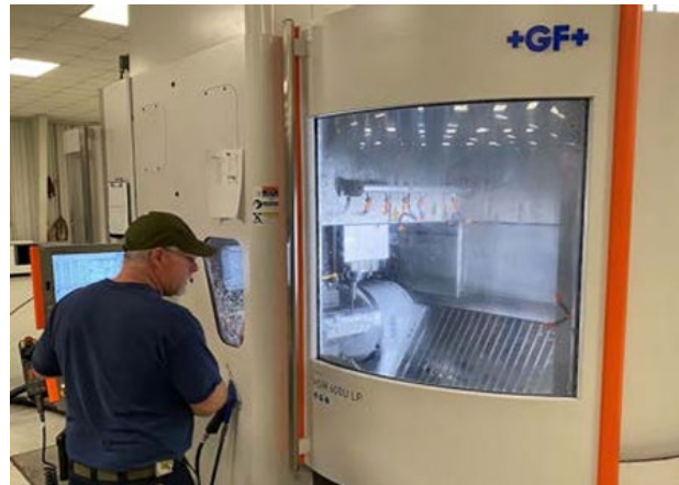
Machine operator checking operation of Gray's DMG 5-axis machining center, with one of company's three Mazak 5-axis machining centers running unattended in the background.
