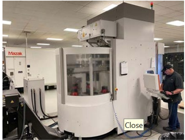
Machinist checking operation of Gray's DMG 5-axis machining center, with one of company's three Mazak 5-axis machining centers running unattended in background.
