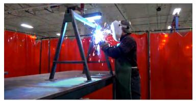
Not only is TIG a cleaner process, it provides welders a greater chance to be artistic. With TIG, welders have full control over the amount of heat and the penetration level of the bead. They can also start and stop in any position and don't have to worry about impurities.
