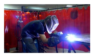
Also referred to as Gas Metal Arc Welding (GMAW), MIG -- an abbreviation for Metal Inert Gas -- is a semi-automatic welding process that feeds a consumable, which is the wire, onto the workpiece. TIG, which stands for Tungsten Inert Gas, and can sometimes be called Gas Tungsten Arc Welding (GTAW), is a manual welding process that uses a non-consumable tungsten electrode to produce the weld.
