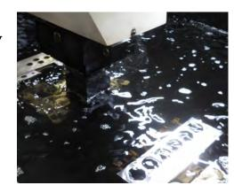
Unlike other types of machining, EDM creates a desired shape by using an
