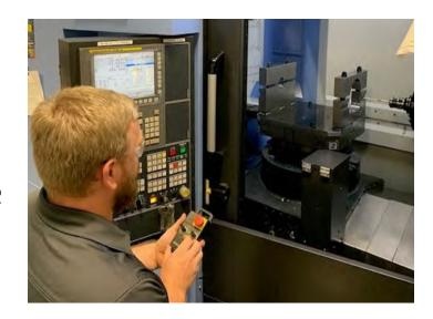
Also commonly referred to as horizontal milling, horizontal machining is the process of removing metal from a workpiece with rotary cutters oriented horizontally. Unlike its more popular cousin vertical machining, horizontal machining has the spindle parallel to the ground floor with the tool sticking out and cutting across the side of the workpiece.
